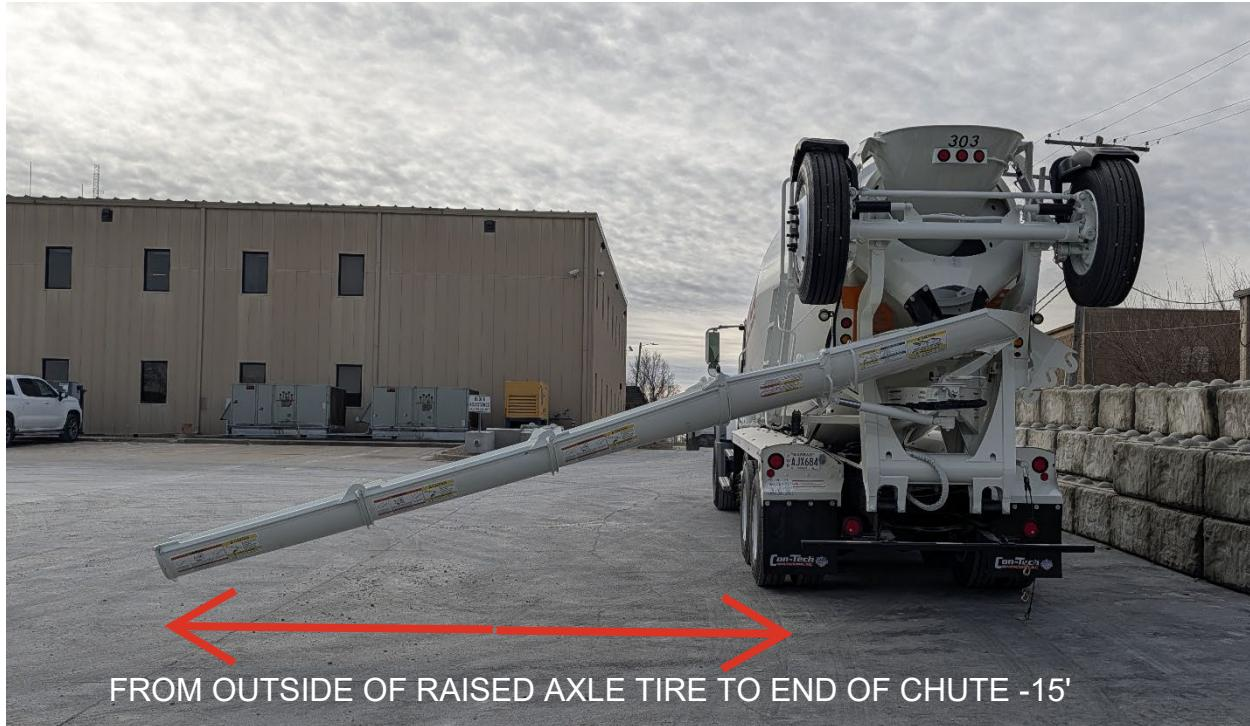
FROM OUTSIDE OF RAISED AXLE TIRE TO END OF CHUTE -15'
